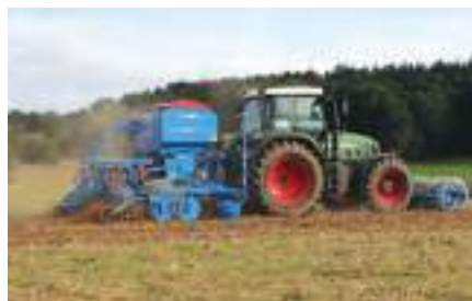
Lemken Solitair 9 series drill working with a front-mounted press.
