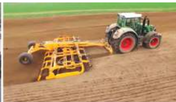
Seedbed preparation in one pass - Agrisem's Vibrogerm.
