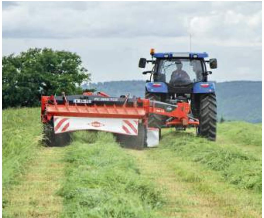
Centre pivot attachment on some Kuhn mowers allows cutting on either side of the tractor.
