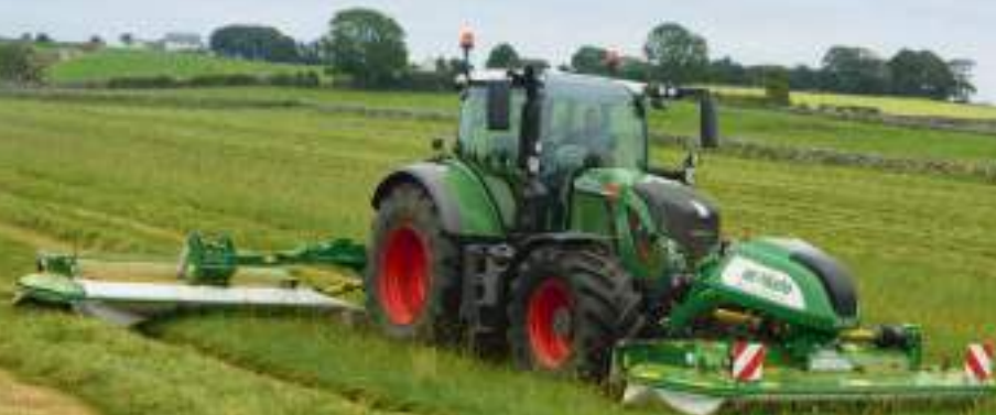
The front and rear-mounted McHale Pro Glide mower-conditioners have a 3.1 m wide cutterbar.
