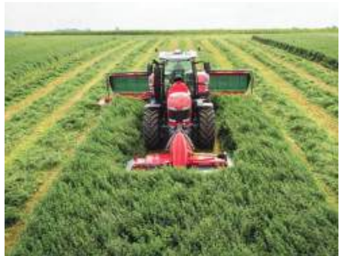
Massey Ferguson front and rear-mounted mower-conditioner combination with three 6-disc cutterbars.
