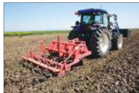
Maschio Pinocchio subsoilers are available with three, five or seven tines with 45 cm maximum working depth.
