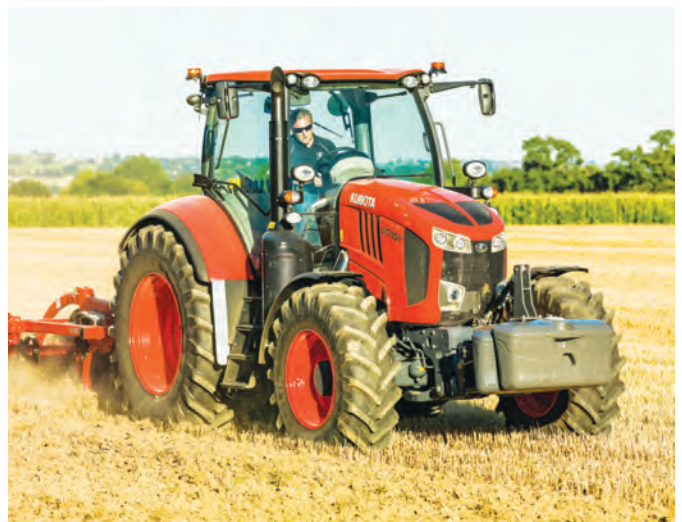
Kubota M7001 series tractors are built in France with up to 175 hp maximum power output.
