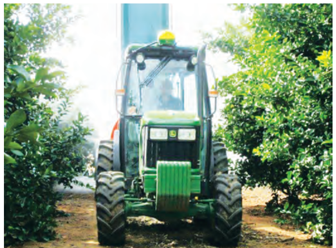
The John Deere 5E series utility tractors have power outputs between 55 and 75 hp.
