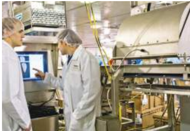
Computer vision technology has proved to be some of the most empowering technology ensuring in-process product quality and safety. Georgia Tech has developed these innovative computer vision system screens to detect individual meat and poultry portions online for both volume and visual quality.
