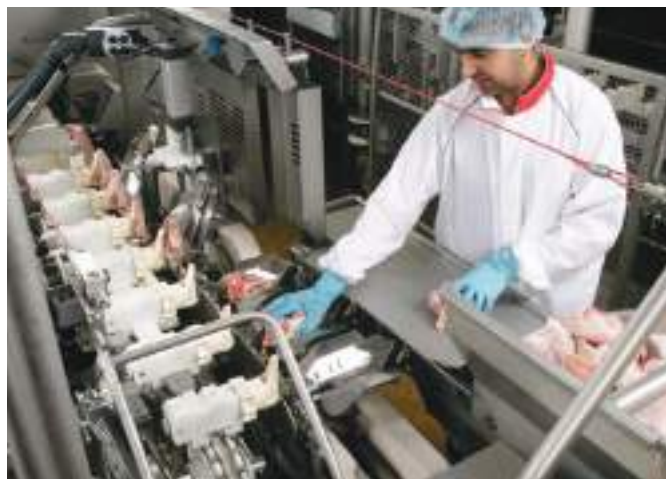
AMF-BX FlexControl, by Marel/Stork Poultry Processing, the modular breast cap deboning system that produces a wide variety of high yield fillet products.
