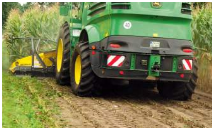
Kemper's The StalkBuster allows for controlling corn borer without plant protection agents. (Photo: Kemper)
