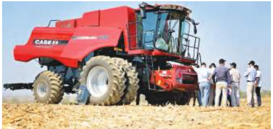
Case IH's AF7140 combine harvesters featuring advanced Axial-Flow single rotor technology on display at the show. (Photo: Case IH)
