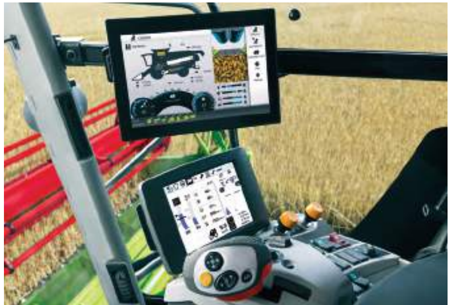
Cemos Auto Threshing – automatic threshing control for CLAAS straw-walker and hybrid combine harvesters. (Photo: CLAAS)
