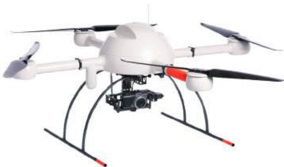
This md4-1000 from Microdrones is equipped with a multispectral camera that can deliver data on humus content, the irrigation condition or stone and weed content at the surface.
