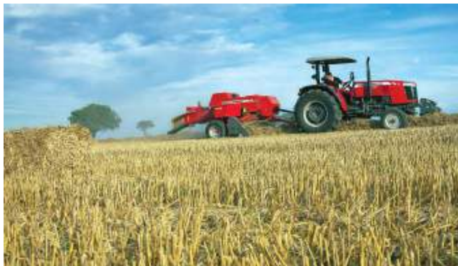
Massey Ferguson's MF 1840 small baler has the pick-up reel in line with the bale chamber.
