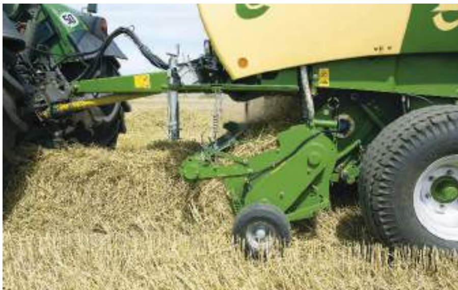
A Krone Comprima round baler equipped with the EasyFlow cam-free pick-up reel.
