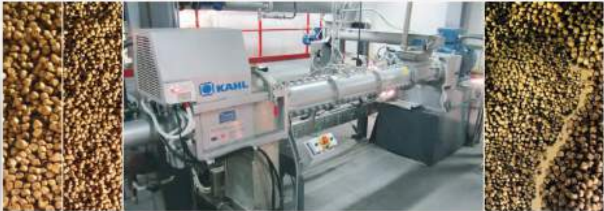
Contrary to conventional extruders, the KAHL extruder OEE is equipped with a hydraulically adjustable die.
