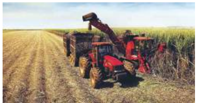
Case IH Austoft 8800 sugar cane harvesters and a Puma 240 tractor during harvesting operations.
