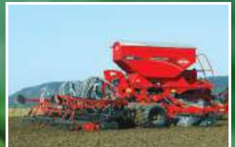
A 6.0m wide version of Kuhn's Speedliner pneumatic drill for reduced cultivation systems.
