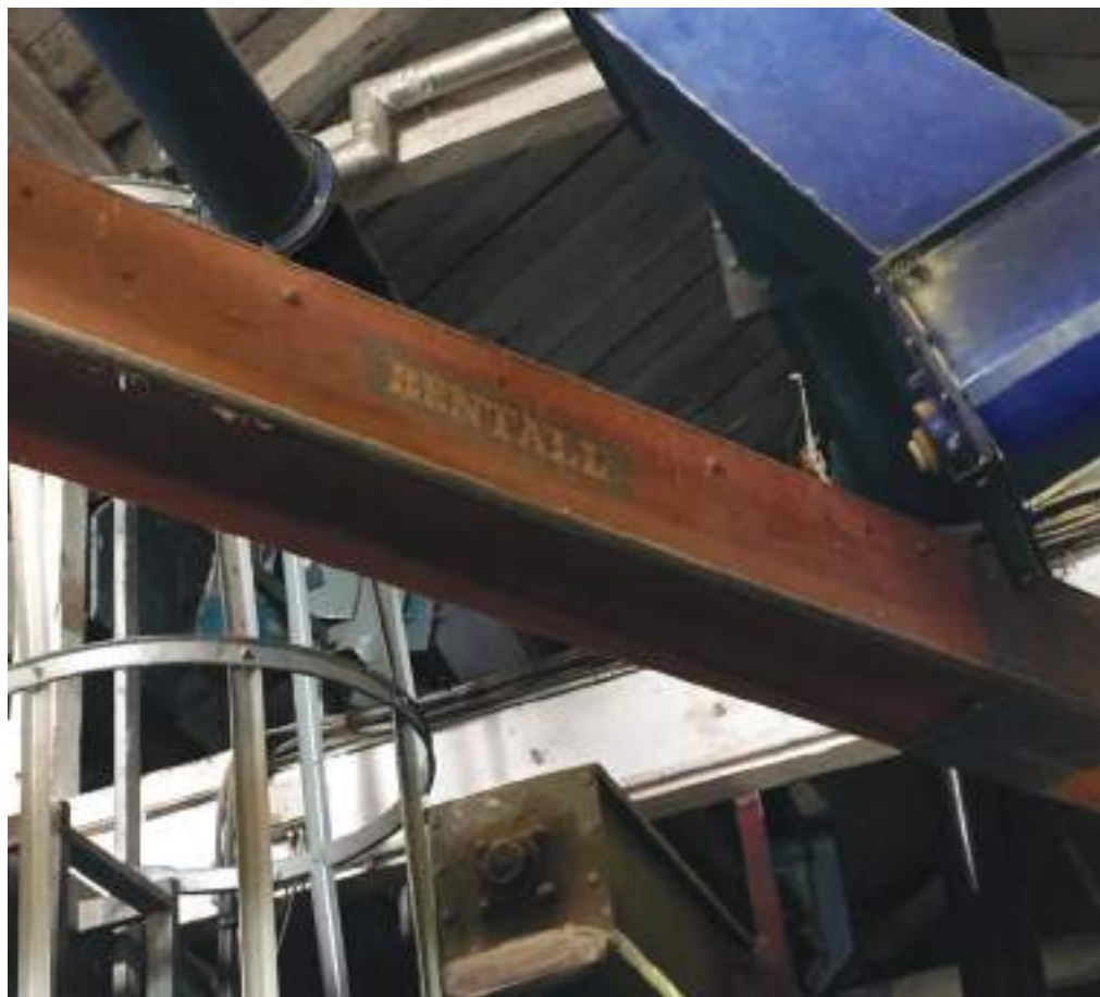
A wooden chain and flight conveyor which was installed in the 1950's and is still used today in a Bental Rowland silo. (Photo: Bental Rowland)
