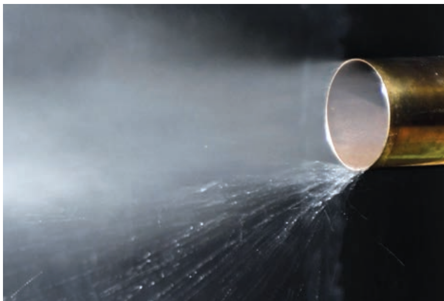
Standard fogging tube flow rate 27 litres per hour with nozzle 1.2
