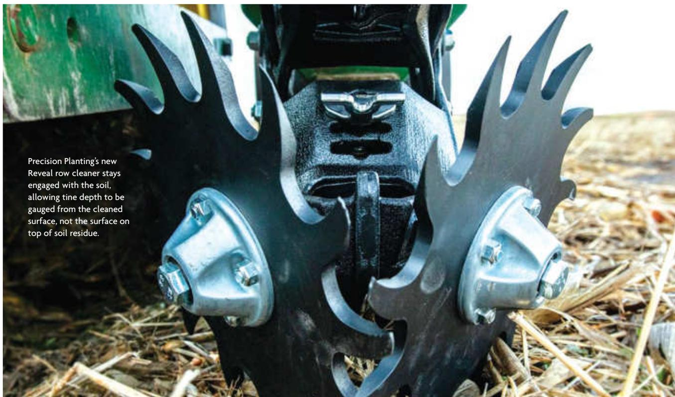
Precision Planting's new Reveal row cleaner stays engaged with the soil, allowing tine depth to be gauged from the cleaned surface, not the surface on top of soil residue.
