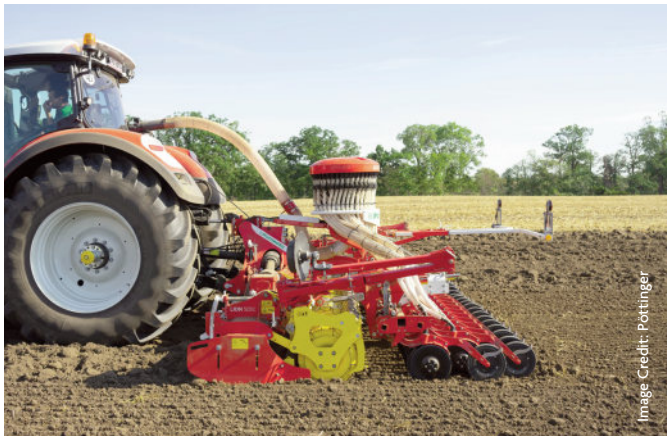
Both LION models operate with four rotors per metre of working width.
