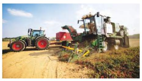
The machine uses optical sorters to harvest fruits and vegetables. (Photo: Volvo Penta)
