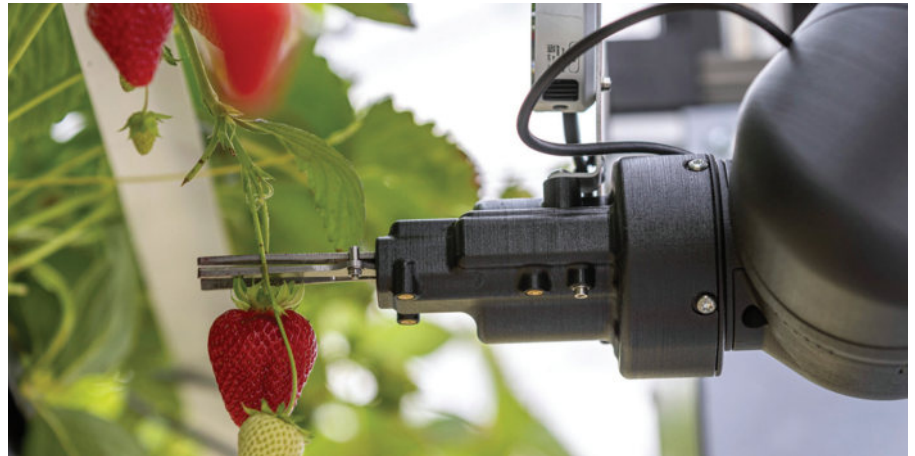
The robot's arm, equipped with a camera and a patented gripping system, uses cloud computing and artificial intelligence to locate the strawberries, determine their degree of ripeness and place the ripe fruit safely in a basket.
