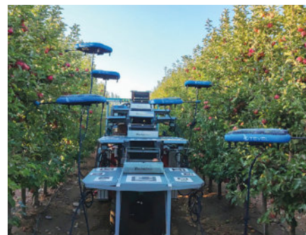
Tevel's Flying Autonomous Robots harvesting apples in Unifrutti's orchards in Linares, Chile.
