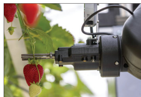
The robot's arm uses cloud computing and AI to locate strawberries, determine their degree of ripeness and place the ripe fruit safely in a basket.
