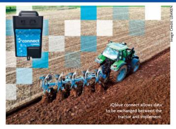
implements. The module is connected to the tractor via its ISOBUS interface. It also features GPS and a mobile data connection for communication, for example with a farm management system. The system automatically adapts to the implement it is connected to at any time and therefore substantially reduces the user's workload.
