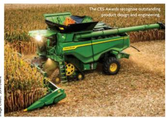
The X9 1100 is the largest John Deere X Series combine and helps farmers harvest faster without risking grain loss or quality. These machines can thresh, separate, and clean more bushels per hour, or harvest more acres per day, even under unpredictable conditions. Compared with previous models, the X9 1100 can harvest up to 70% more wheat per hour.
