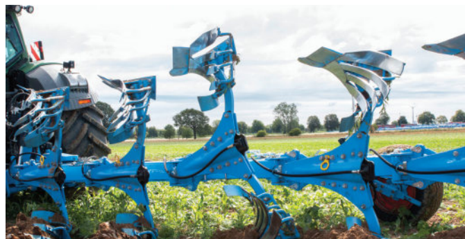
The new overload protection OptiStone at the LEMKEN Juwel 10.
