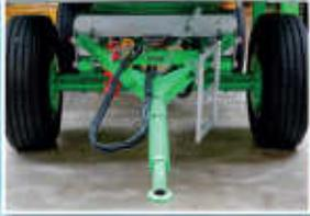
**Y-shaped drawbar for easy manoeuvring**
