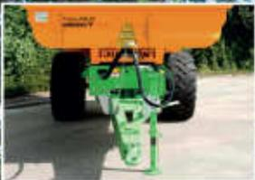
**Large open drawbar to keep a very good weight/strength ratio**
